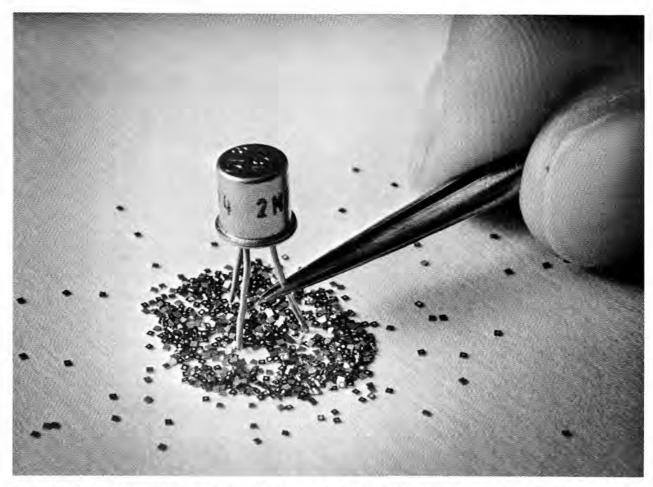
ONE METHOD of miniaturizing components is to eliminate bulky containers. Here a standard transistor bestrides serveral hundred transistor chips. A single chip in a hybrid circuit typically performs the same function as the large transistor in the container.
